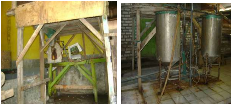
Gambar 7. Kondisi Eksisting Disc Mill & Wash Tank di Ponpes Sunan Drajat, Paciran - Lamongan
