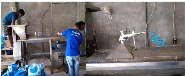
**Fig. 2.** The testing of brush water spray using a compressor. (left)
