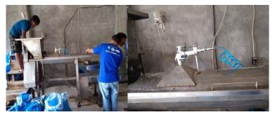
Fig. 2. The testing of brush water spray using a compressor. (left)Fig. 3. The position of the brush water spray that was put into the screw of iodized machine (right)
